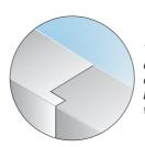
Two wall panels are attached with an indentation, ensuring that inner and outer joints are on different levels. The panels are attached by welding or bolting, enabling installation in locations where welding is not possible.
