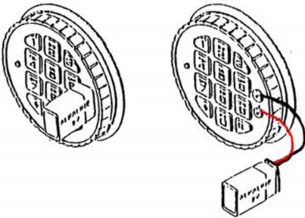
If the batteries have not been changed in time and the tension does not suffice to cancel the lock's blocking feature, a new 9V **ALKALINE** battery can be pressed onto the contacts on the entry, until the code has been entered and the entry is rotated. When Time Delay is programmed, use a battery clip (on general sale). Black upper position, red lower position.
