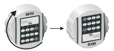
If the input unit is turned back to its starting position in anti-clockwise direction after the five-second ready-foropening period, the lock will return to the blocked position and can only be unblocked after renewed clearing and reentry of a valid code.
